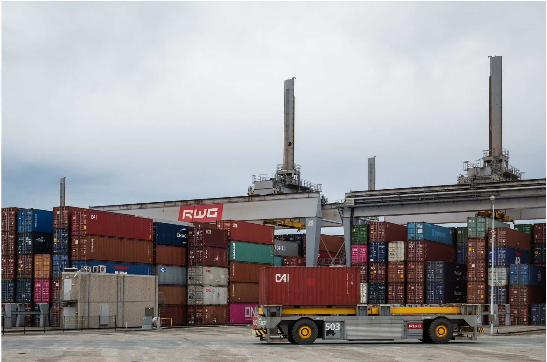
Rotterdam. An automated, self-driving container transporter at the Rotterdam World Gateway (RWG), a cutting-edge area developed recently in the western part of the port.
