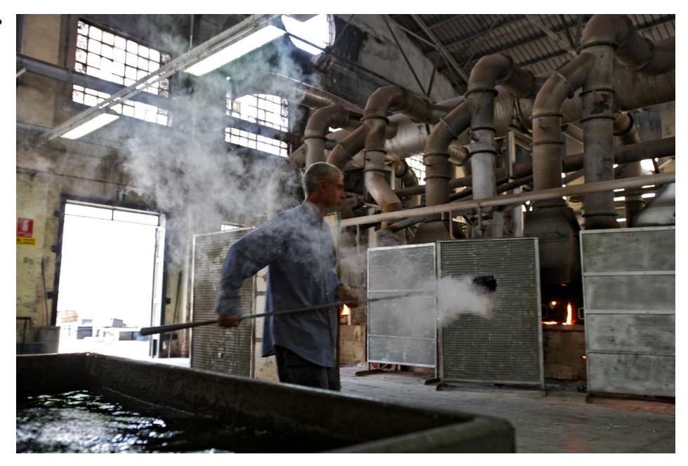
Cooling of the glass block from which the glass canes will be pulled. Effetre factory in Murano (Venice) is the only one that still produces glass canes for processing glass beads.
