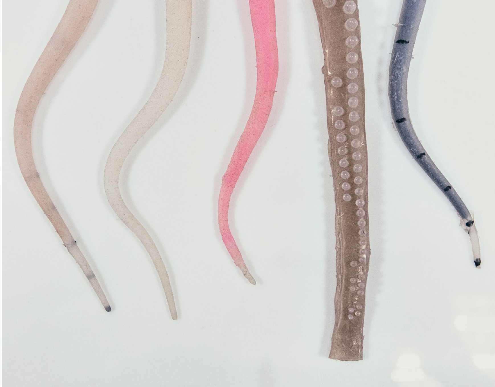
Pontedera (Pisa), Sant'Anna School of Advanced Studies. Robotic arms in soft materials bio-inspired by octopus tentacles. The soft robots are created with soft, flexible materials, inspired by nature, capable of interacting safely with man and the external environment. The school has a multi-disciplinary approach bringing together in a single research institute robotics experts, botanists and mathematicians as well as specialists in material sciences, design and IT.
