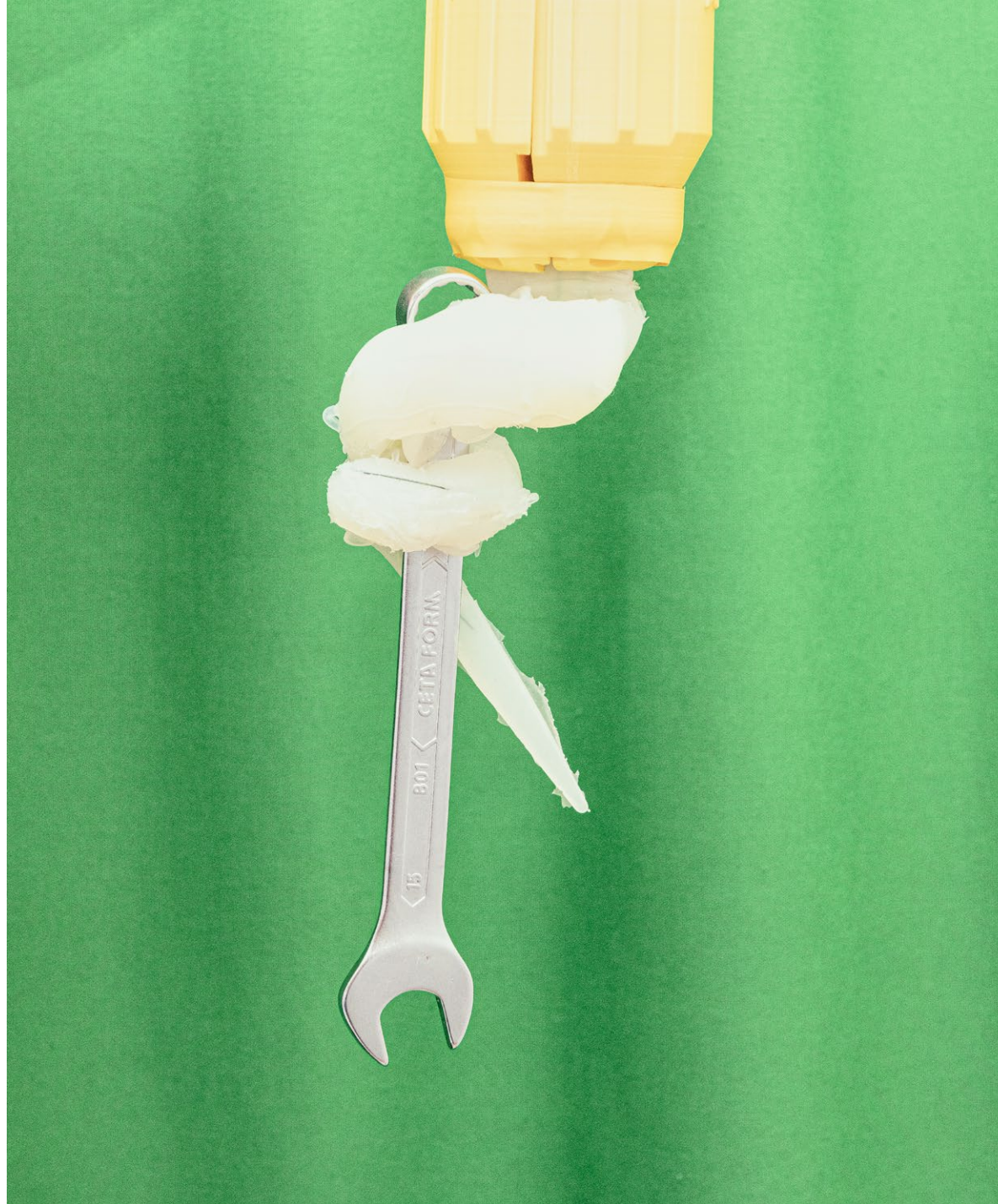
Pontedera (Pisa), IIT, the Italian Institute of Technology. A robotic tentacle to retrieve objects from inaccessible places such as oil wells. The bio-inspired arm of the octopus can grasp shapes that are not easy to pick up, such as a spanner.
