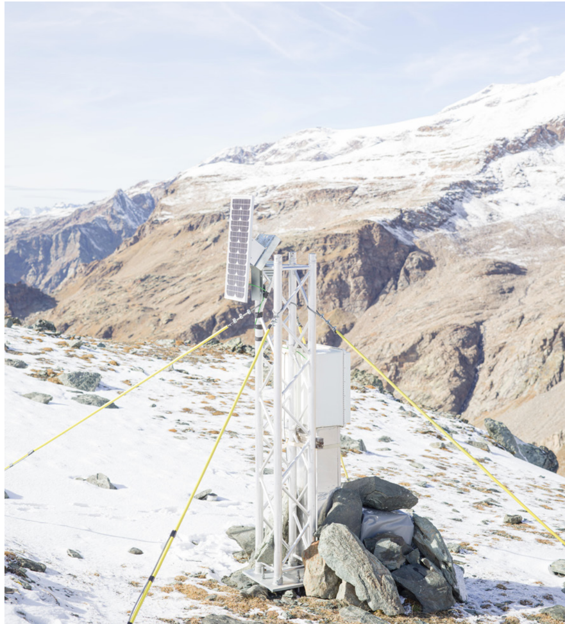
The instrumentation that's used to collect data, such as the piece of equipment shown in the photo positioned on the summit of the Corno del Camoscio mountain in the Monte Rosa massif, must withstand high winds, lightning and extreme weather conditions.
