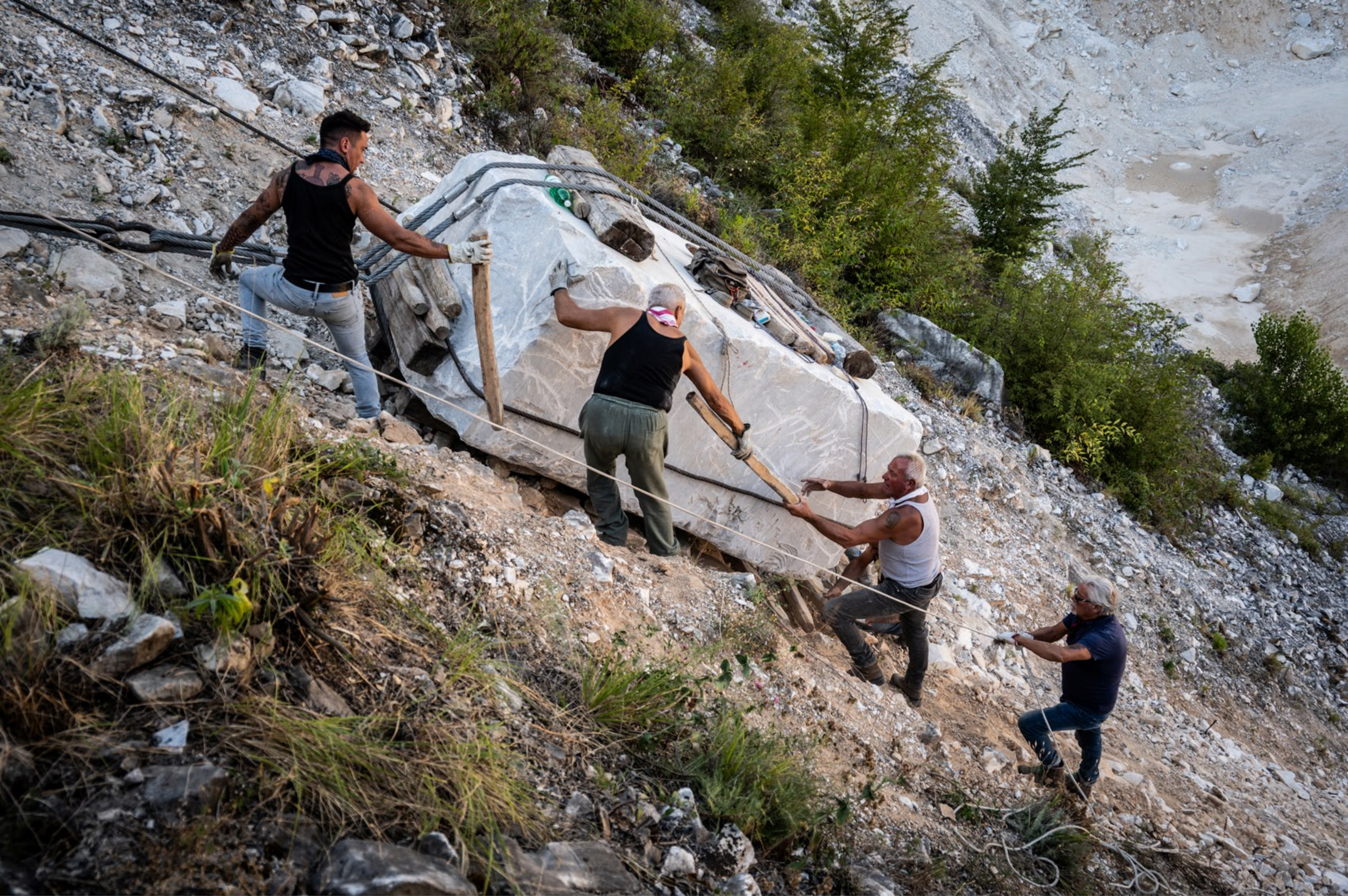
Bridges of Vara (Carrara, Italy), a moment of "historical lizzatura," the reconstruction of how the very heavy marble blocks were slid from the quarries by hand, only through the use of cables, ropes and lumber.
