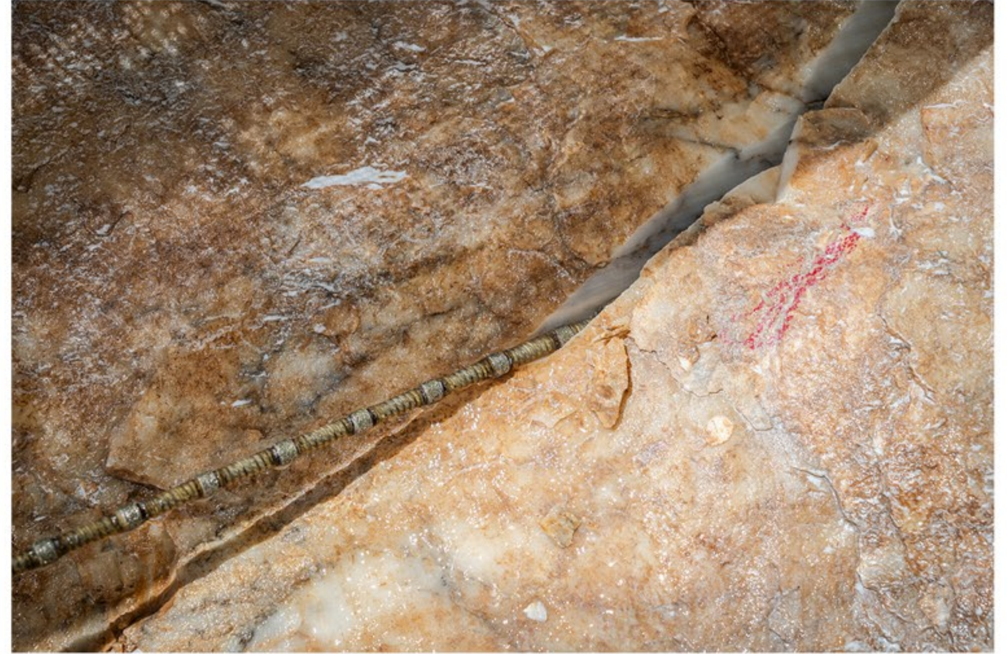
A diamond wire cuts marble in the Cervaiolo quarry in Seravezza, Lucca (Italy).
