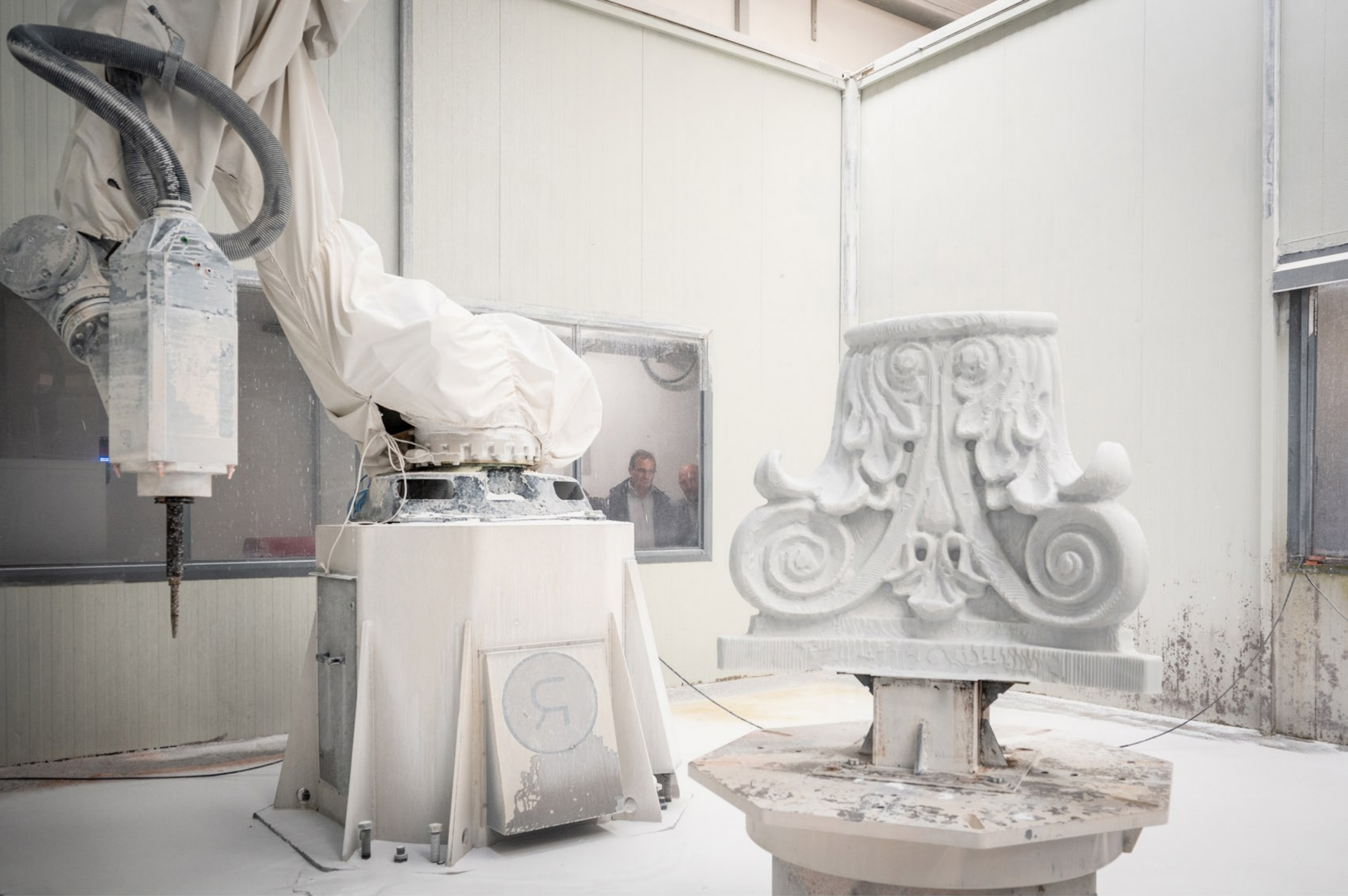
Querceta (Lucca, Italy), in the laboratories of the Henraux company two technicians observe the final result of a white Carrara marble capital made by a robot sculptor.
