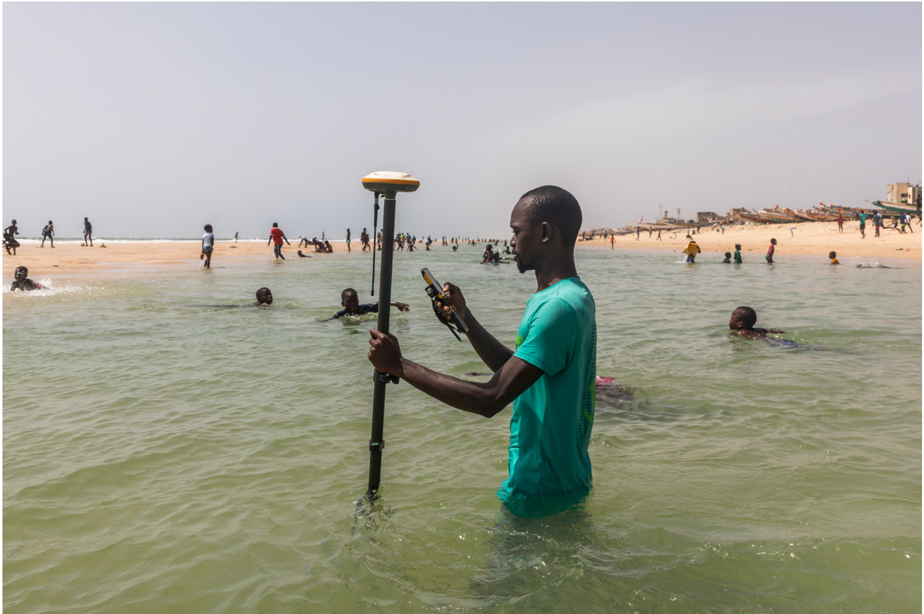
Senegal, St. Louis – Kobe, a young PhD student from Dakar University, is conducting geological surveys to monitor sea level rise along the Langue de Barbarie, the narrow strip of land located between the ocean and the Senegal River.
